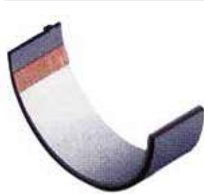
Two-component bearings For low to medium loads in gasoline and naturally aspirated diesel engines in passenger cars—consisting of a steel support shell, an intermediate layer, and a layer of bearing metal (mainly aluminum alloys).
