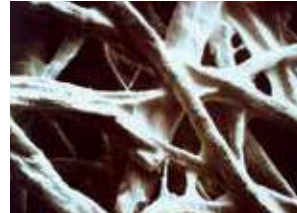
The impregnated cellulose fibers under a microscope.
