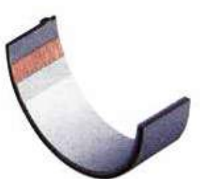
Three-component bearings Built from a steel support shell, bearing layer, barrier layer, and an overlay—for use in highly loaded engines. Their performance is improved by “sputtering,” which increases hardness, load capacity, and wear resistance. Sputter bearings are intended for super-charged engines with charge air cooling and are also increasingly found in passenger car diesel engines.
